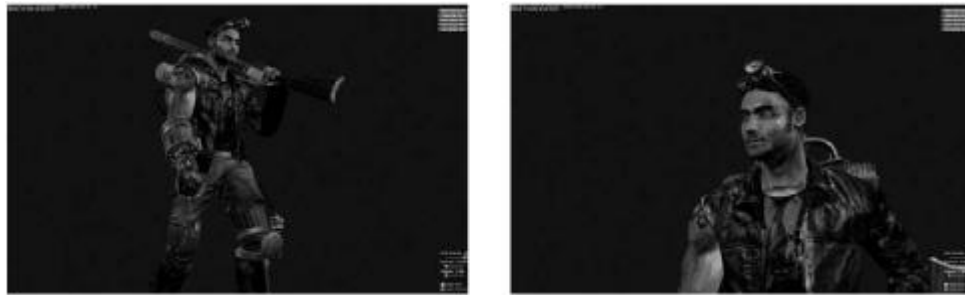
Figure 1.4.9. Screenshots showing our algorithm in action. We saw about 8.9 fps for the view on the left and 15.1 fps for the view on the right on the ATI Radeon 5870. Increase in the frame rate was due to view frustum culling patches.
