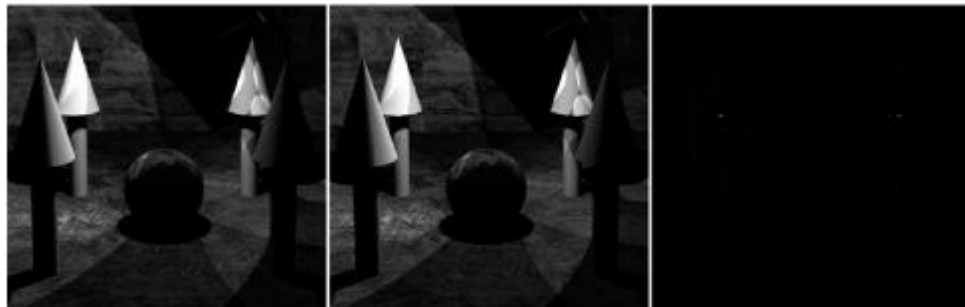
Figure 1.3.1. Deferred shading (left: 20 fps), multi-resolution deferred shading (center: 38 fps), and their difference image (right). There are 40 spot lights, including fuzzy shadows (1024×1024 pixels with 24 shadow samples per pixel).
