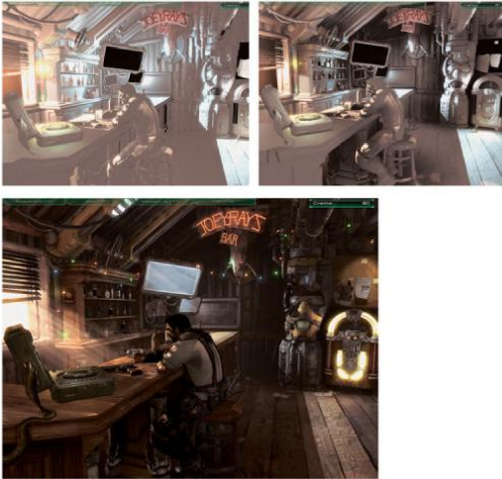
Color Plate 2: Comparison of large- versus small-area SSAO samples from Gem 1.2. The images show the contrast between the large-area, low-contrast SSAO sampling component on the bar surface and background in the image on the left and the tighter, higher-contrast SSAO samples apparent within the helmet and nooks and crannies found on the character's space suit in the middle image. Final output is on the right.
