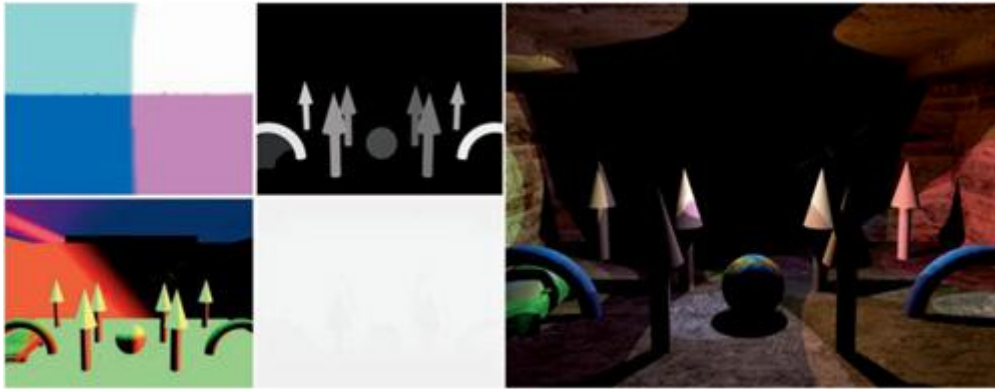
Color Plate 4: The deferred shading technique presented in Gem 1.2 has three steps: geometry pass, multi-resolution rendering pass, and composite pass.
