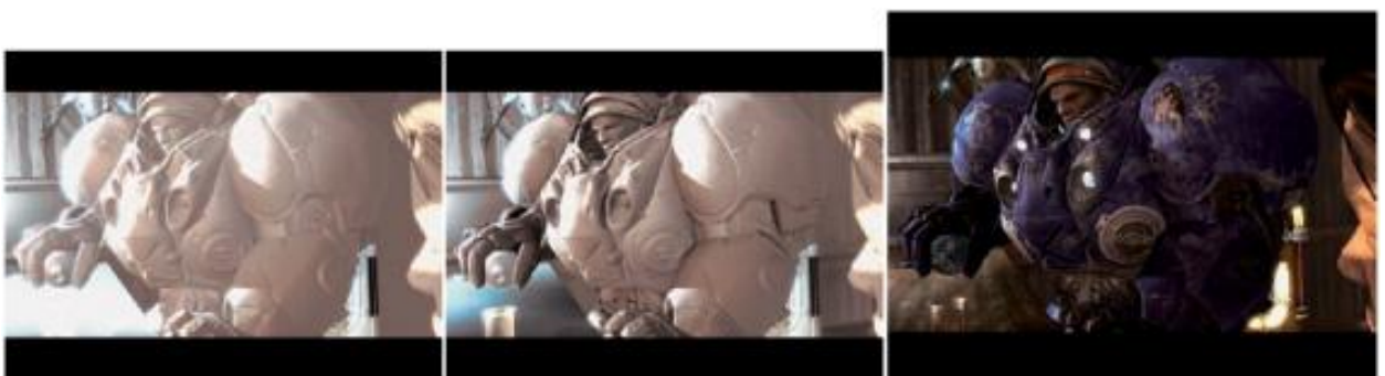
Color Plate 3: Output of rendering stages and final image from the deferred rendering technique described in Gem 1.3. Position and material ID (top left), normal and depth G-buffers (bottom left), and a resultant image (right).
